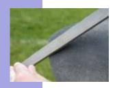
Next we need to sharpen those tools. Shovels, hoes, axes and trowels are easily sharpened with a hand file. An 8 inch long mill file with a bastard cut will do the trick nicely. First secure your tool with a vise or other method to keep it from slipping away from you. Hold the mill file at the same angle of the previous sharpened blade and push the tool across the edge. Do NOT push back and forth; just push away from you in one direc-
