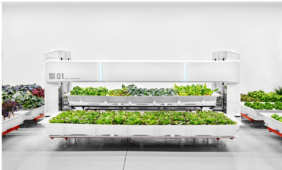
Angus navigates the farm and moves the 4ft.x8ft. hydroponic systems to the robotic arm for various operations
