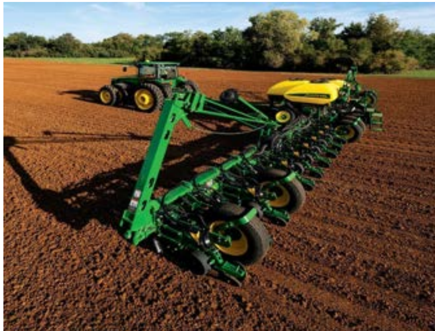
John Deere "ExactEmerge" Planter - 300+ years after Jethro Tull's Seed Drill
