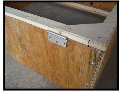
Step 4. (optional) Attach wood triangles to lid corners to stabilize the lid when using light weight cover materials.
