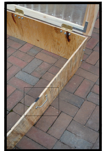
Step 5. Attach a handle to each side of the box.
