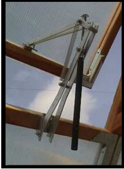
The temperature activated lift mechanism is a convenient way to control the internal temperature of the cold frame.
