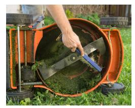
Grass can become tangled around the blades and impede the blade. Remove and sharpen the blade to have it ready for next spring. It is a clever idea to oil the blades to prevent any rust from forming. You have two choices; drain the oil and replace now or leave until spring and change the oil. It is an innovative idea to always leave oil in the engine. Texas has such a mild winter, the choice to change the oil in fall or spring is your option.
