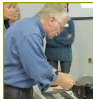
Bill removes the burr edge as the final touch using the wet grinding stone.
